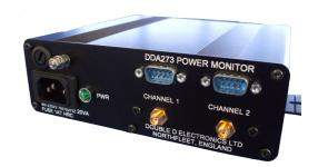
The DDA273 is a dual-channel RF level monitor, able to signal when the level on each RF input is outside preset limits. It accepts a wide range of input signals, and is able to discriminate at levels approaching -50dBm.
