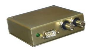
Double D Electronics Ltd can offer a range of IF amplifier blocks in both  $50\Omega$  and  $75\Omega$  configurations, with a variety of gain options. Each amplifier includes fault monitoring (based on power supply current), with two relay contact outputs.
